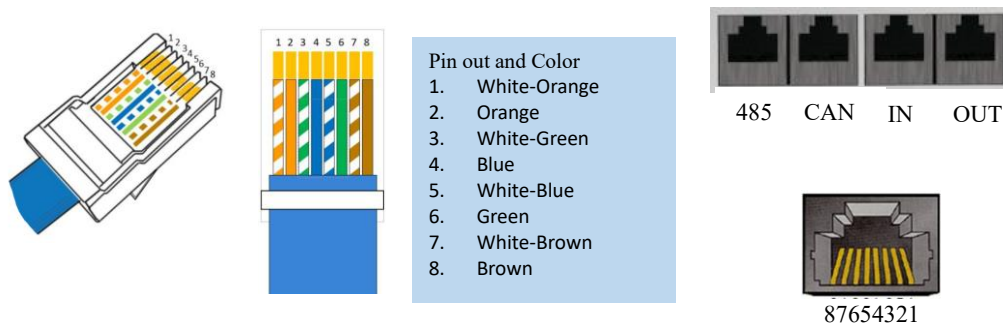
Figure 2-2 CAN,RS485,OUT,IN interface definition
